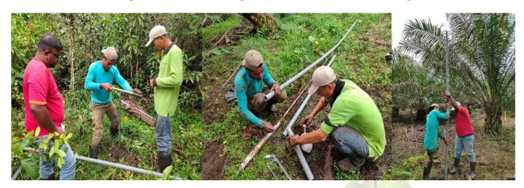
Figure 1. The pictures illustrating the piezometer installation process at BBEFR including the measurement of peat depth and installation of piezometers
